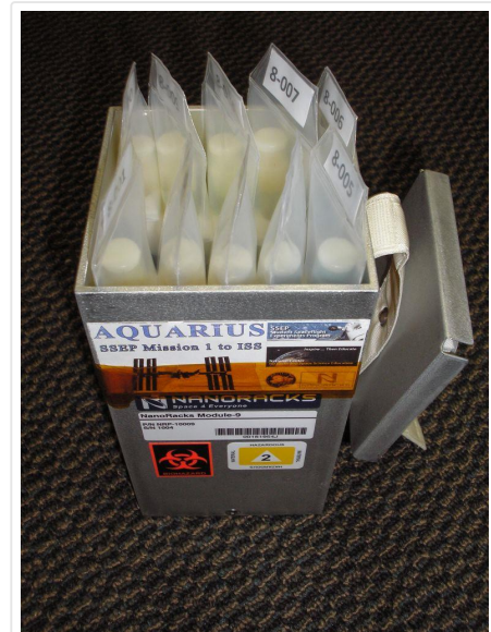
Figure 6: SSEP Payload Box containing FME Mark 2 mini-labs. CLICK ON IMAGE ABOVE FOR ZOOM
