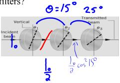
How can light be transmitted through "crossed polarizers?"
