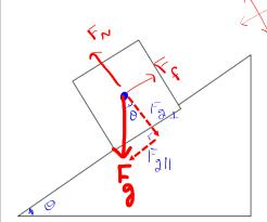
Resolving  $F_{\rm g}$  into components that are parallel and perpendicular to the surface of the inclined plane:
