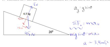
6. Calculate the force of friction acting on the box if it now accelerates down the incline at a rate of 0.67 m/s<sup>2</sup>.
