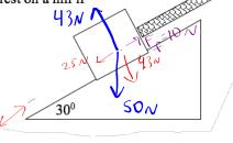
4. Calculate the tension in the rope when this 50. N box is being dragged up the hill at a constant speed of 5.0 m/s if there is a 10. N frictional force acting on it.
