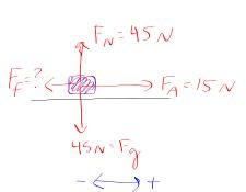
b) Determine the coefficient of friction.
