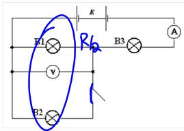
b) State what effect closing the switch has on the total resistance and total current as well as the current through each bulb and the brightness of each bulb.
