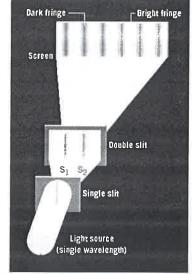
In a double slit experiment, light whose wavelength is 6.0 x 10<sup>-7</sup> m is shone through two slits that are 0.10 mm apart onto a screen that is 2.5 m away. What is the distance between the central maximum and the first bright band?
