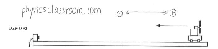
Sketch below your predictions and the results for the fan-cart moving towards the detector and speeding up at a steady rate.
