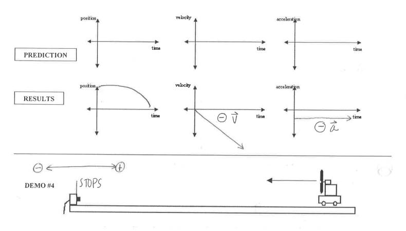
Sketch below your predictions and the results for the fan-cart moving towards the detector and slowing down at a steady rate.
