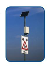
A solar cell produces electricity by using light energy from the sun. Solar cells are useful for things that need electricity but are not near an electrical outlet. States like New Mexico and Arizona use a lot of solar cells because they have a lot of sunlight, and many desert areas are far from electricity.
