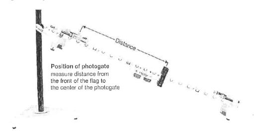
1. Place the car at the top of the ramp. Place the photogate 10 cm down the hill from the car. Measure the distance from the front edge of the car's flag to the middle of the screw that holds the photogate to the track. If you line up the car's flag over one of the
