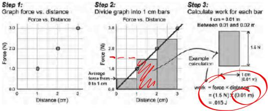
d. To get the total work done on the car you need to add up all the work done as the rubber band straightens out and moves the car forward. Use the table below to calculate the work done.
