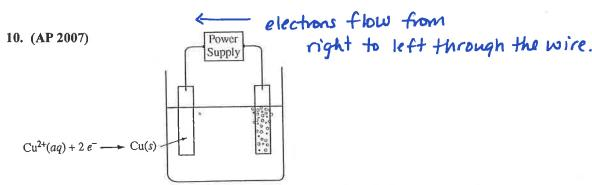
An external direct-current power supply is connected to two platinum electrodes immersed in a beaker containing 1.0 M CuSO<sub>4</sub>(aq) at 25°C, as shown in the diagram above. As the cell operates, copper metal is deposited onto one electrode and  $O_2(g)$  is produced at the other electrode. The two reduction half-reactions for the overall reaction that occurs in the cell are shown in the table below.
