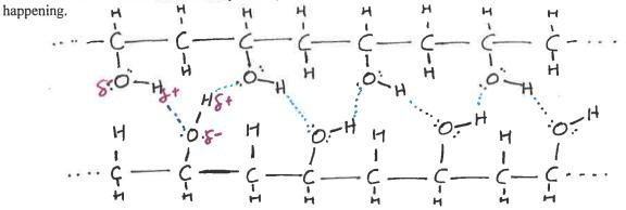
Borax Cleaner contains Na<sub>2</sub>B<sub>4</sub>O<sub>7</sub><sup>·</sup> 10 H<sub>2</sub>O (sodium tetraborate decahydrate). Boron compounds can dissolve in water and react to form a variety of "borates", including  $BO_3^{-3}$ ,  $B_2O_5^{-4}$ ,  $B_4O_7^{-2}$ , and  $B(OH)_4^{-1}$ When a solution of borax is added to a solution of polyvinyl alcohol (PVA), the borate ions increase the attractive forces between the polymer chains.
