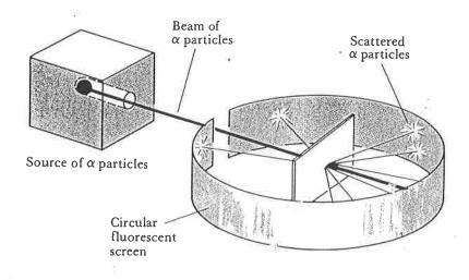
**Experiment:** Rutherford shot positive particles called alpha particles at a thin sheet of gold foil. The foil was surrounded by a screen coated in zinc sulfide, a material which glows when hit by high energy particles, such as the alphas.
