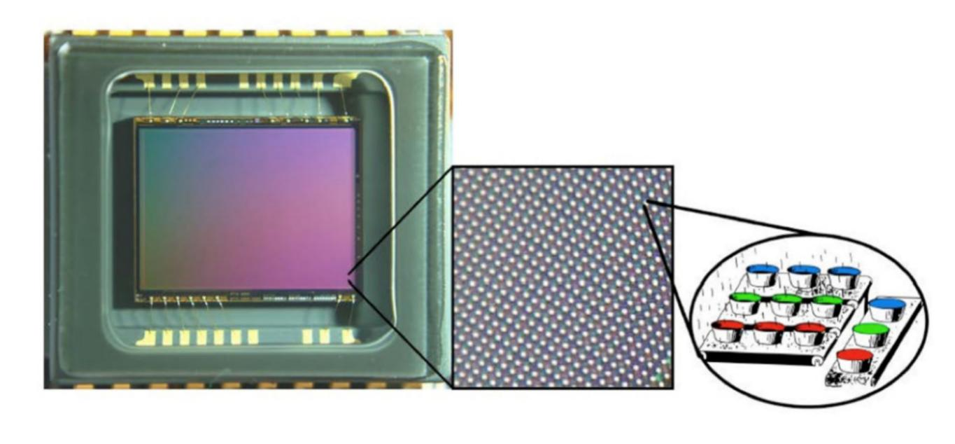
The white lines in the enlarged image are very thin electrical wires that take electrical signals from the CCD to the miniature computer that is in every digital camera.
