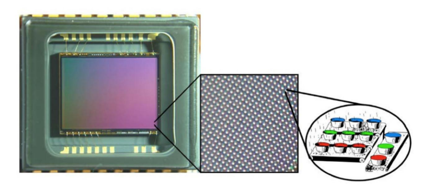
In reality, there are no microscopic cups on the CCD—the surface is flat—but the artist felt that the cups would provide a visual to explain that there are small circular areas that are sensitive to light.
