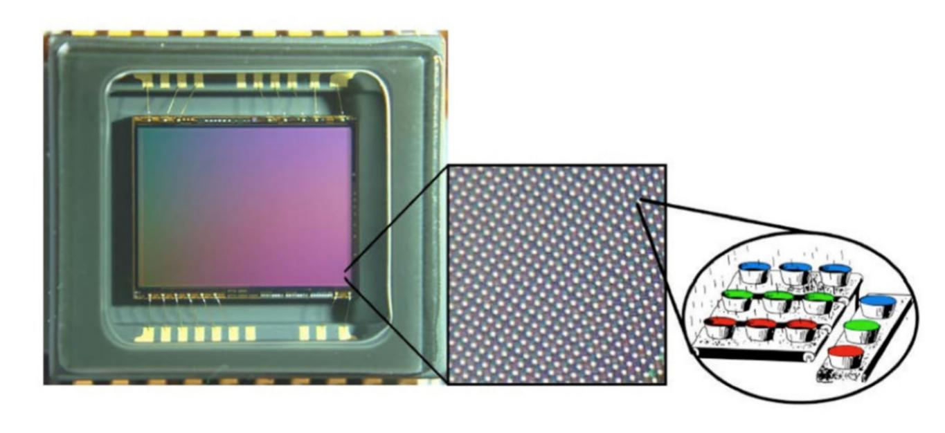
Just like there are three types of cones in the retina, there are three types of light sensors on the CCD. The CCD was made to simulate the way the human
