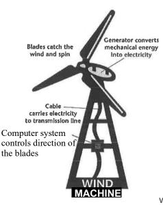
← Horizontal-axis wind machines are more common because they use less material per unit of electricity produced. About 95% of all wind machines are horizontal-axis. A typical horizontal wind machine stands as tall as a 20-story building and has three blades that span ~60 meters (200 feet) across. The largest wind machines in the world have blades longer than a football field! Wind machines stand tall and wide to capture more wind.
