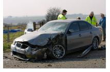
This BMW has obviously suffered a severe impact and appears extensively damaged. However, none of the damage was to the passenger compartment -- the front crumple zone did its job. TIM GRAHAM/<u>GETTY IMAGES</u>
