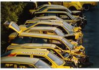
These cars have been put to the collision test at an automobile safety research facility in Wolfsburg, Germany. Notice how the crumple zones appear to have absorbed most of the impact. PETER GINTER/GETTY IMAGES
